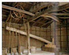
Sake-brewing equipment: press
